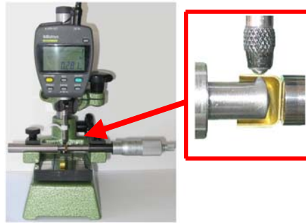
Fig. 5: Measurement of wall thickness depending on the angle to rolling direction and cup height (for better representation shown with a halved cup), similar devices exist for bottom end radius area
