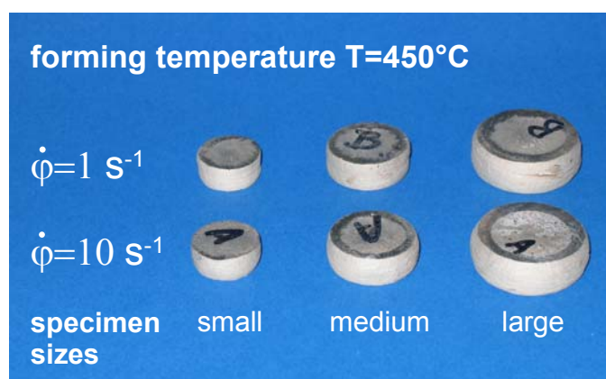
Fig. 6: Illustration of homogeneously compressed specimen at 450^{\circ}\text{C} forming temperature
