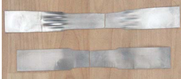
Fig. 2: Wrinkling and failure at conventional tension test of thin sheet (thickness 0.1 mm)
