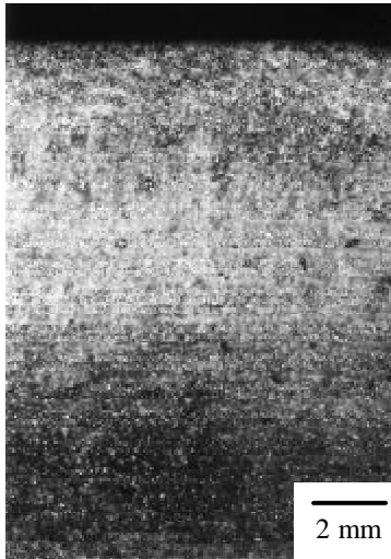
Figure 2. Longitudinal section of a gradient material with 30 – 70 vol% \text{Cr}_3\text{C}_2 (I)
