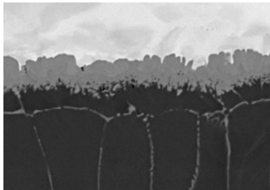
Fig. 5 Backscatter electron microscope picture of a St14/AA6xxx-joint.
